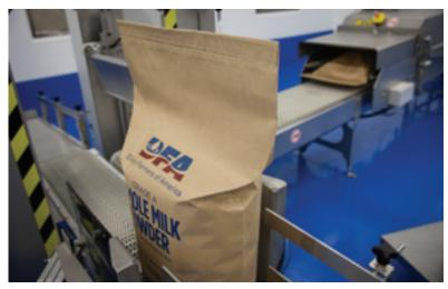
■ Employees at DFA's new milk powder plant in Fallon, Nev., can fill six 25-kilogram, oxygen-free bags of powder every minute. These are trucked to Oakland, Calif., and loaded on container ships bound for China and other countries.
